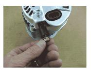
1. Remove 3 screws holding rear cover and then remove cover.
